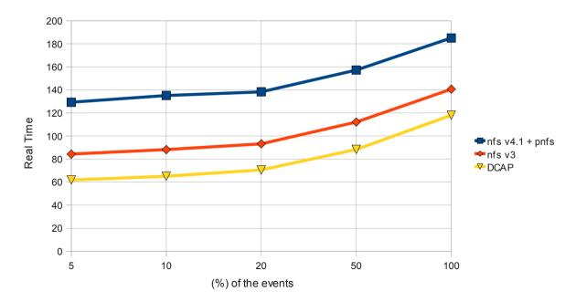
While the test turned out to be irrelevant it have shown that with nfsv3 client send less read requests than with v4.1.
