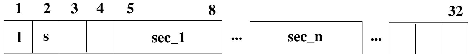
first four octets: length octet,  $l = 4 * n$ , (n: size of the array of the security mechanisms),
